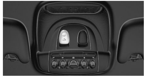
SOS button in the roofliner
